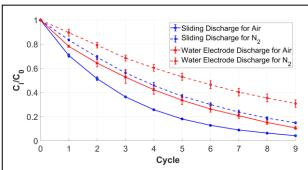
Fig. 1.: Relative concentration of Rh-B over multiple treatment cycles for sliding discharge and water electrode discharge using air and  $N_2$  as the working gas
